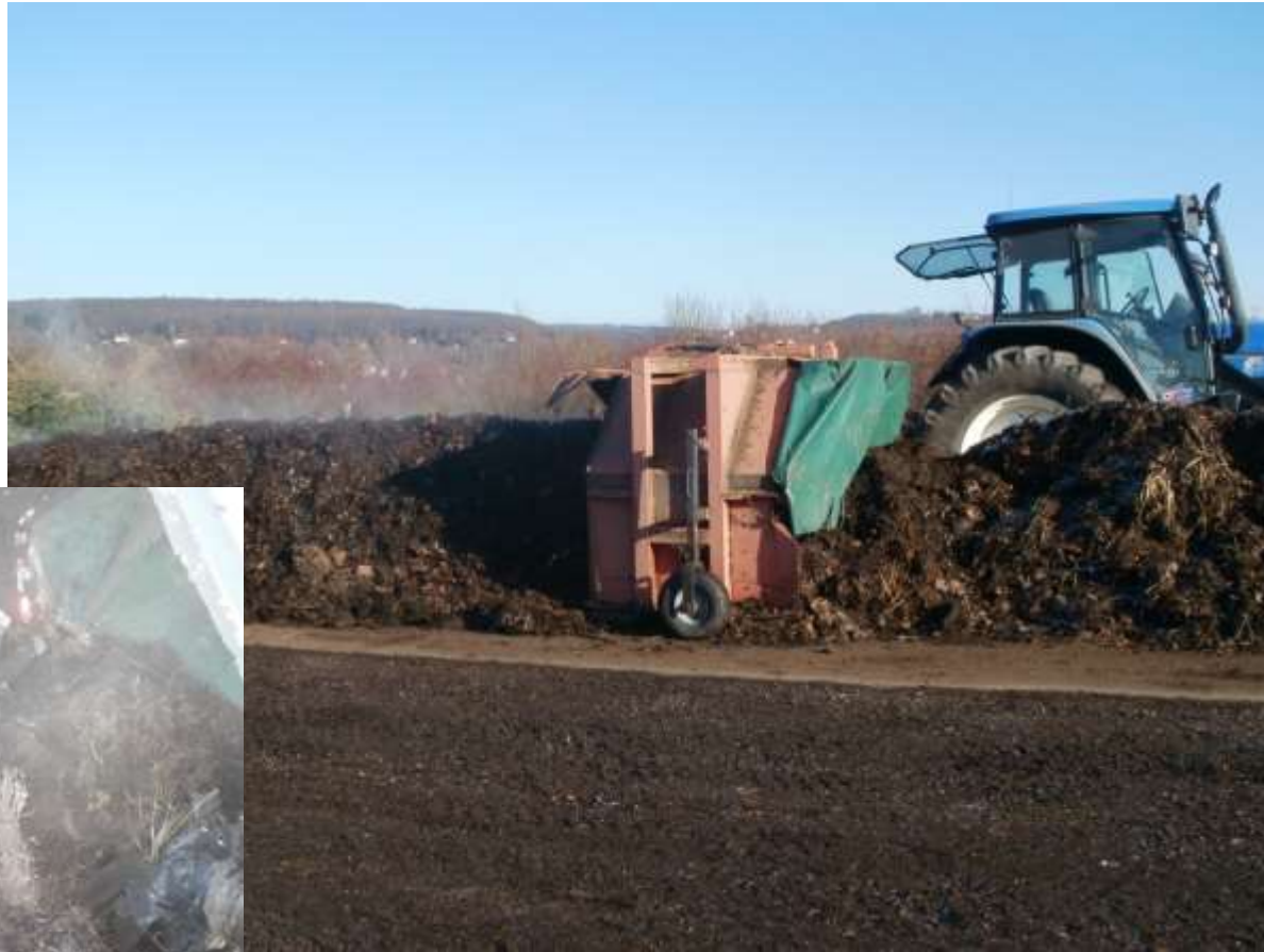
Small compost turner for rows with 2,5m wide and 1,8m high, turning wave inside
