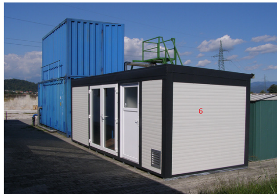
Picture: Biomethane modular unit (number 6 ) – container with adsorbent vessels (Pressure Swing Adsorption – PSA) and computer controlled electronic measuring system for continuously measuring physical and chemical properties of biogas and biomethane
